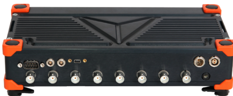
Rear side connectors of the analog-out version
