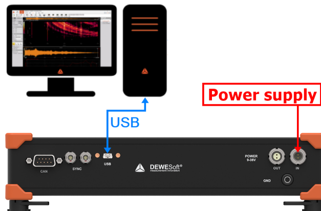
SIRIUS USB: connectors on the rear side
